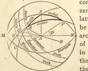
complement of that altitude or the zenith distance of the sun; let de zenith distance of the sun; let the latter be represented by z. Let  $\phi$  be the latitude of the place, or the arc NP. Let  $\delta$  be the declination of the sun or the arc QS. Then in the spherical triangle PZS, the three sides are known, and hence the angle Z can be found from the
